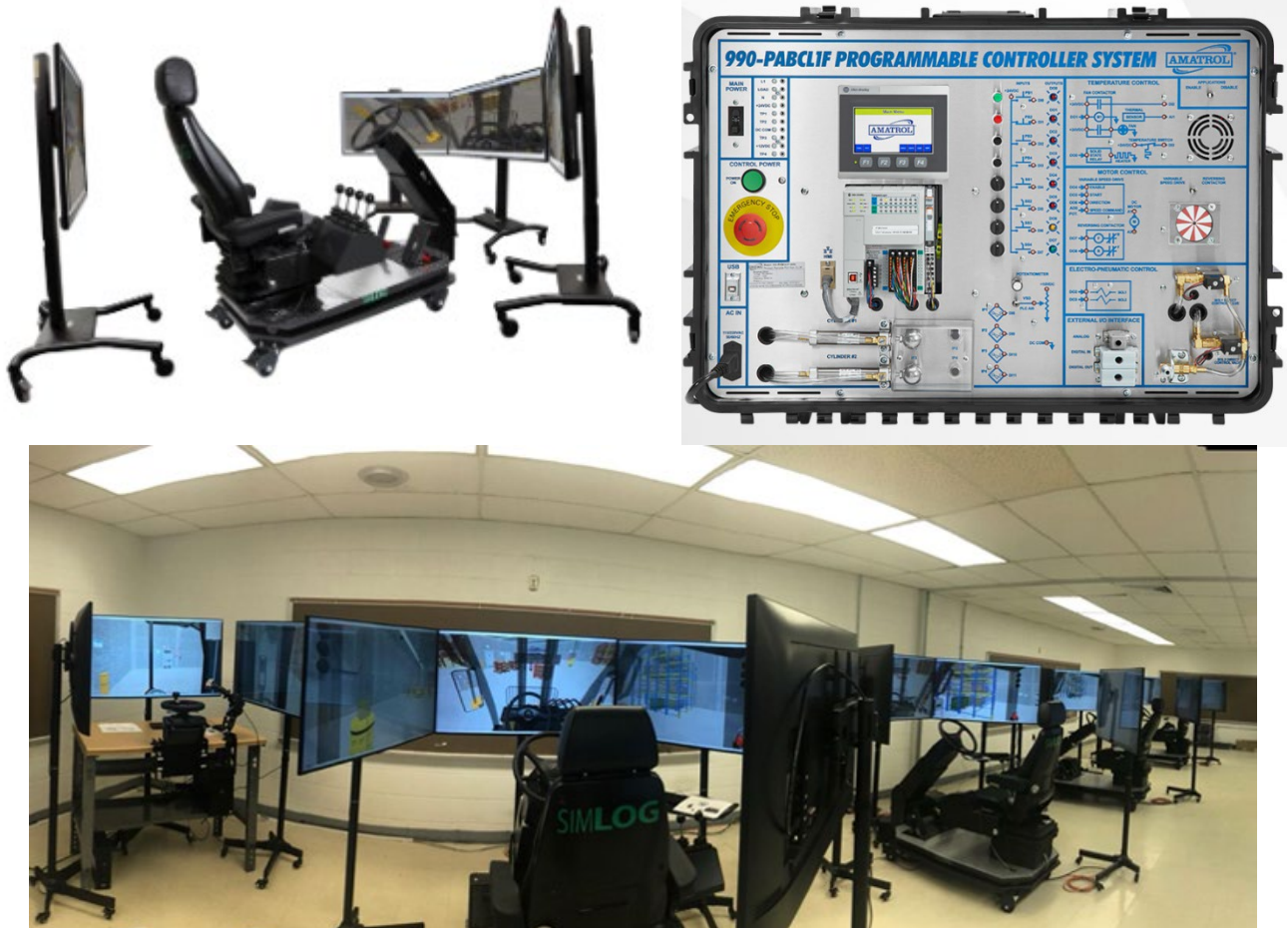
Image of the Simulator used for Heavy Equipment Operator training
